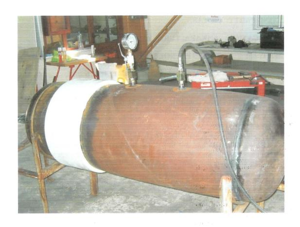
AT PUMP LIMIT, PRESSURE OF 137.5 BARG REACHED. STRONGBACK REPAIR SEEN CONTAINING EXPANSION AS UNWRAPPED PORTION OF PIPE SHOWN BALLOONING.
